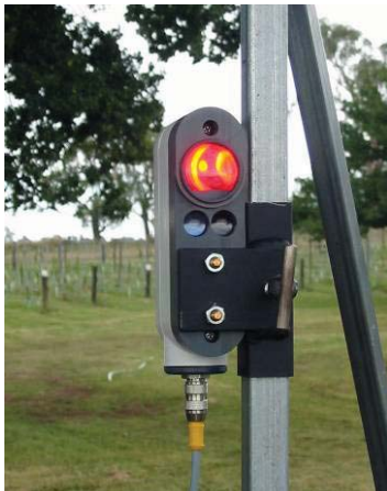
Photograph of the CropCircle (red) unit showing pulsing LED's located in the top of the detector head (note, only red radiation emitted by the LEDs is visible) and dual photodetectors below.
