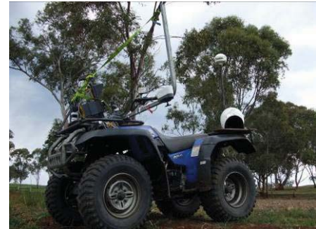
ATV-mounted CropCircle (with GPS and datalogger) for on-the-go surveying.
