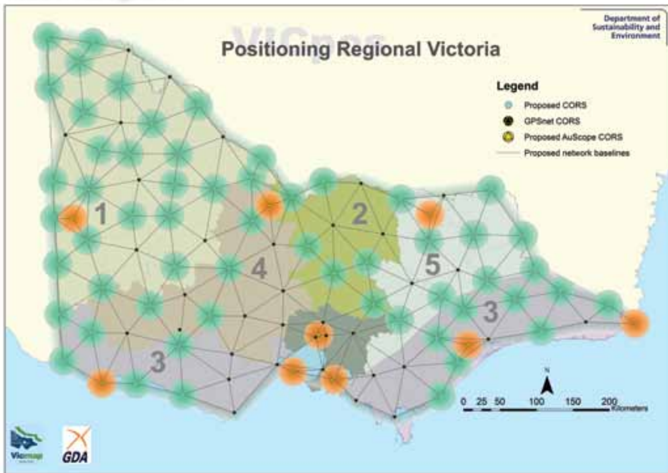
Figure 1. Position Regional Victoria project – the expansion of GPSnet GNSS CORS network over the coming months and years.
